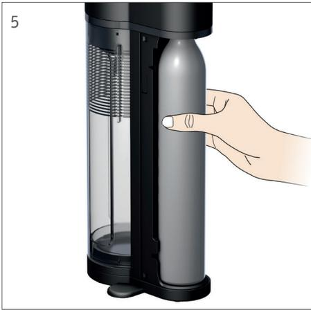
**7** Swing open the safety door to the left. Ensure that the CO<sub>2</sub> lance is tilted forward and locked in place. Push the bottle filled up to the mark completely upwards over the CO<sub>2</sub> lance. Then push the bottle backwards towards the carbonator until it is aligned vertically. Briefly pull on the bottle to check.
