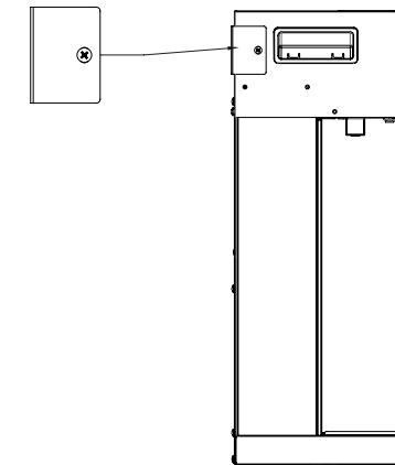
**2.1B** Decide on a stable wall and mount the mounting strip in the position where you want to hang the electric fireplace. After aligning the bracket, mark five drill holes on the wall. Drill the five holes for the appropriate dowel size that you want to use for mounting purposes.
