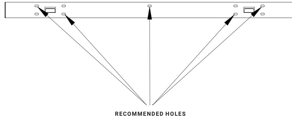
**2.1C** Push the plastic dowels into the five drill holes. Then fix the mounting strip to the wall using five ST5 x 40 screws.
