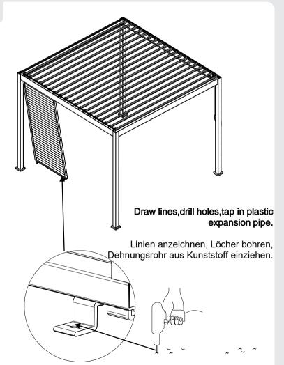
If the floor is a wood floor, you don't need to knock in the plastic expansion pipe, directly use J to knock in the floor.
